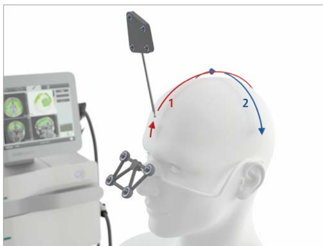
Manually controlled calibration: steps 1 (red) and 2 (blue)
